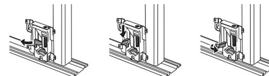
**A Rotate** anti-jump clip into open position
