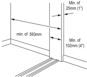
To reduce your opening width by up to 127mm / 5" on each side use Spacer Blocks together with the end fillet and appropriate infill. Detailed instructions are provided with each Spacer Block pack.
