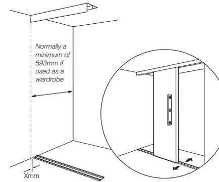
**Floor Track** - Position the track on the floor of the opening. Mark where holes need to be drilled in the track (we recommend a fixing at each end and centre then at regular intervals in between). Before permanently fitting the floor track to your floor, fit the door into place and using a spirit level adjust the Floor Track so the door becomes vertical.
