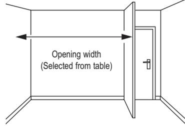
To stop the doors short of an obstruction such as a window or door, construct a return end panel from melamine faced chipboard. Cut to fit the exact ceiling height and scribe back edge to fit rear wall and skirting. Fix return end in position with Fixing Blocks equally spaced.
