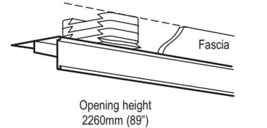
For ceilings between 2399 - 2729mm / 94 1/2" - 107 1/2" use Opening Reducers. Detailed fixing instructions are provided with each Reducer pack.
