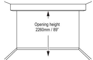
If your ceiling height is between 2272 - 2399mm / 89 1/2" - 94 1/2" use Spacer Block to reduce it to 2260mm / 89". Detailed instructions are provided with each Spacer Block pack.
