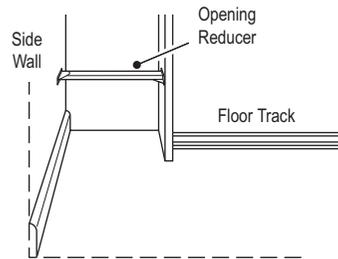
To reduce your opening by more than 457mm / 18" on each side you can construct an 'L' section using an end panel and end fillet. Jointed together with Fixing Blocks and scribed to fit the wall and skirting.
