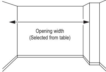
To reduce your opening width from between 127 - 457mm / 5 - 18" on each side you can use Opening Reducers fixed to the side wall. Detailed instructions are provided with each Opening Reducer.
