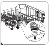
To remove the upper spray arm, hold the nut in the center still and rotate the spray arm counterclockwise to remove it.
