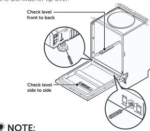
The maximum adjustment height of the feet is 50 mm.
