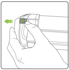
Release the latch with the green arrow, to pull open the bin lid.
