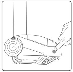
Rest the AirRam K9 on its side and locate the brush bar button on the right hand side. Press the button inwards and then pull the brush bar out from the bottom of the AirRam.
