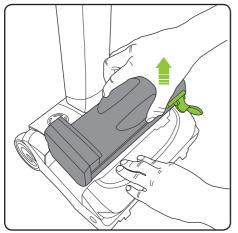
Holding onto the AirRam K9 with one hand, pull the bin handle and lift the bin out of the AirRam.
