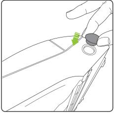
To get the best performance on hard floors with deep crevices remove the brush bar as shown on page 12. Insert the supplied brush bar hole plug into the side of the head assembly as shown in the image above.
