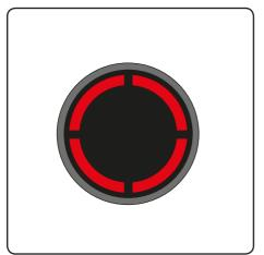
If the brush bar jams during use, the AirRam K9 will stop and the LEDs will appear red. You will need to remove and clean the brush bar (see page 11).
