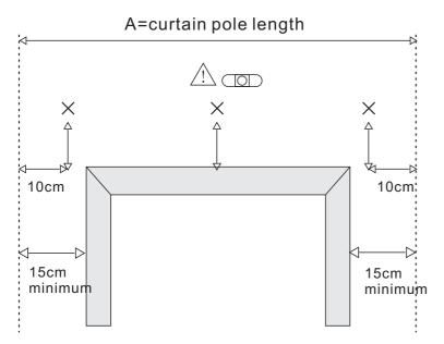
The end brackets must be positioned 10cm in from the end of the pole. If a centre bracket is required, please position this in the centre between the two end brackets. Mark the position on the wall ensuring they are level.
