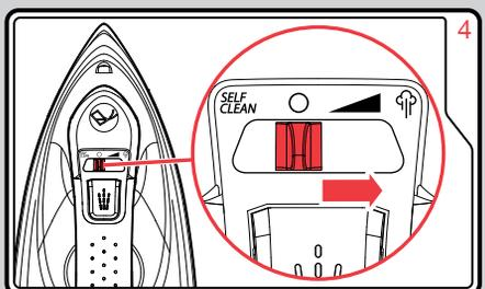
Vary the steam output using the variable steam switch (1), as shown above.
