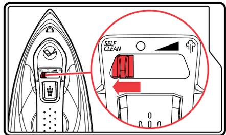
Whilst still holding the variable steam switch in the self clean position, gently move the iron back and forth until the water tank is empty.
