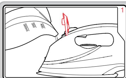
Make sure the iron is not plugged in. Set the variable steam switch (1) to 'O'. Fill the water tank (10) via the filling hole (6). Fill with the iron in a horizontal position to the MAX graphic on the side of the water tank.
