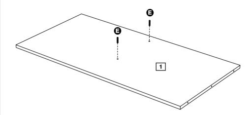
**b:** Carefully place the Table Top Panel 1 onto the unit.
