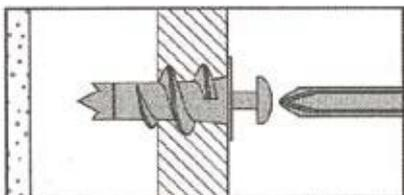
For use when attaching light loads on to plasterboard partitions.
