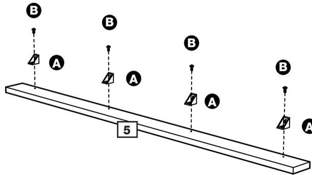
**b:** Use Screws **B** to fix the Front panel **5** onto the Bottom panel **2**.
