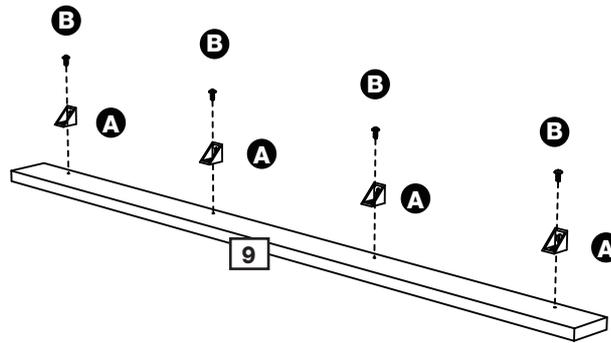
**b:** Use Screws **B** to fix the Front Panel **9** onto the Bottom Panel **2**.
