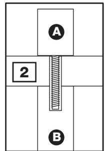
**b:** Fit Bottom Panel **2** onto the unit, then screw in Feet **A**.
