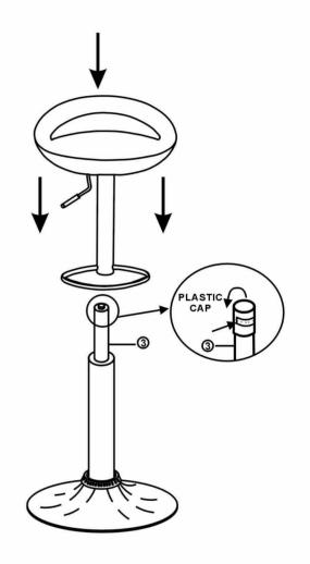
Note: IF the adjuster will not function correctly, remove the seat assembly, and depress the top of the piston to fully extend it. Re-assemble the seat and try adjuster again. |
