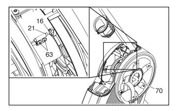
Next, slide the Reed Switch (21) slightly closer to or away from the Pulley Magnet (16), and then retighten the M4.5 x 12mm Flange Screws (63). Turn the Crank Arm (70) for a moment. Repeat these actions until the console displays correct feedback.
