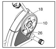
See assembly step 5 on page 7. Using a standard screwdriver, release the tabs along the bottom edges of the Rear and Front Shield Covers (9, 19), remove the two M4 x 12mm Screws (61), and then remove the Rear and Front Shield Covers.
