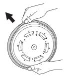
**Removing the gasket:** Pull the rubber gasket from the sides of the inner lid.
