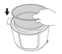
Place the inner pot into the outer body of the pressure cooker.
