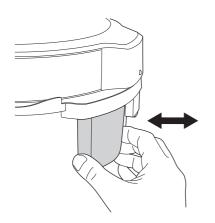
**Condensation cup:** On the back of the steamer under the hinge you will find the condensation cup.
