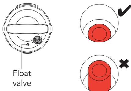
After steam has stopped coming out of the Steam release valve, check that the Float valve has dropped before opening the pressure cookers lid.
