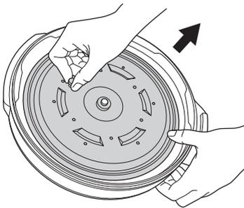
**Removing the inner lid:** Grip the metal peg on the side of the inner lid and pull outwards.
