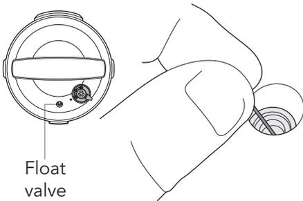
**Cleaning the float valve:** Clean the float valve using a pin to ensure there is no debris trapped inside or around it.
