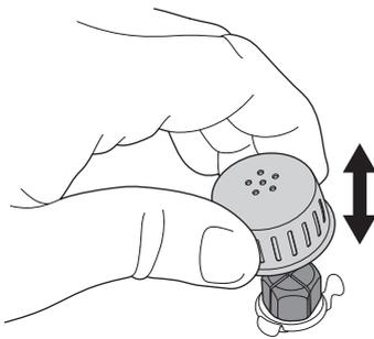
**Cleaning the thimble cover and valve:** The thimble cover is on the inside of the lid and is only visible when the inner lid is removed. Pull the thimble cover off the valve. Use a pin or brush to remove any blockages inside or around the valve and cover. Replace thimble cover by pushing back over the valve. Pushdown until it locks in place.
