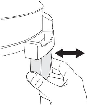
**Condensation cup:** On the back of the steamer under the hinge you will find the condensation cup.
