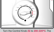
Turn the Control Knob (5) to 200-220°C. The Indicator Light (6) will illuminate. When the oil reaches cooking temperature the light will switch off.
