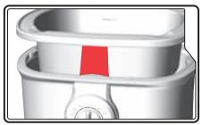
The Thermostat Pad (shown above) is located on the side of the Pan. Greasy deposits in this area cause the Intellichef Multicooker to misread the temperature of the Pan and overheat. When cleaning the Pan ensure the pad is cleaned thoroughly and free of any grease or food deposits.
