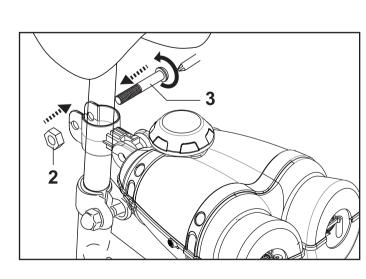
Fasten the screw to fix the bubble exhaust. (spanner not included.)
