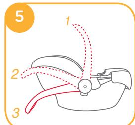
To adjust the handle, squeeze handle buttons on both sides to release it ⑥ -1, and then rotate the handle until it clicks into any of the 3 positions. ⑥ -2
