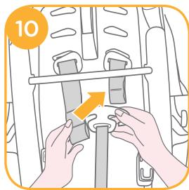
3. Pull the harnesses through the slots in the seat ⑪ -1, and then insert them into the appropriate set of slots. ⑪ -2
