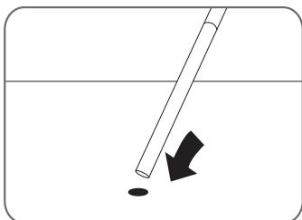
Once the concrete has hardened, insert the airer assembly into the ground socket.
