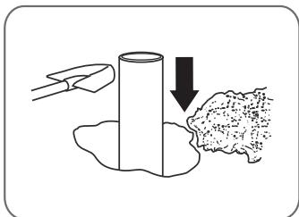
Install the ground socket securely into the ground. **Note:** The ground socket should be installed using concrete (not included); a fence post mix is ideal. Make sure the top of the ground socket is flush with the ground.
