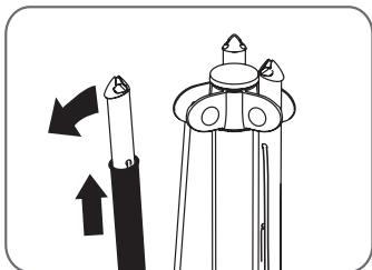
Remove the ground socket from the arm.
