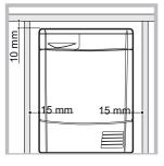
Install the dryer far from gas ranges, stoves, radiators or hobs as flames may damage it. If the dryer is installed below a worktop, ensure there are 10 mm between the upper panel of the dryer and any objects above it and 15 mm between the sides of the machine
