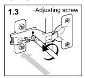
Continue adjustment - see 2 or tighten the fixing screw of the cross plates
