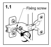
To adjust the door towards the lefthand side - turn the adjusting screw to the right.
