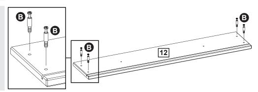
d: Press the drawer front12 onto the drawer sides14
