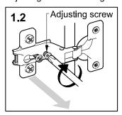
To adjust the door towards the right hand side - turn the adjusting screw to the left.
