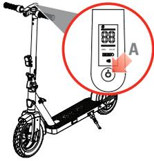
1 The cruise control mode is controlled by the power button on the display (A).
