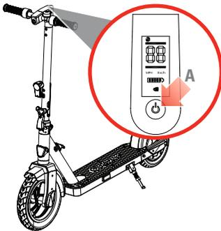
To manually disable the cruise control mode, press the power button (A) quickly four (4) times. The electric scooter will then beep (sound) once and the display will show the letters NC (No Cruise) for a few seconds (E).
