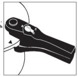
device come visual pressure indicator drops. If secondary safety device come visual pressure indicator has not dropped down after 3-4 minutes use a spoon to press the secondary safety device come visual pressure indicator down. If secondary safety device come visual pressure indicator pops up again, repeat the procedure after waiting for some more time.
