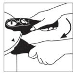
3. Place the pressure regulator on the vent tube in the lid, ensuring that the steam outlet is facing the hole in the lid and that the pointer sits in the recess/notch on the lid handle. Press down gently.
