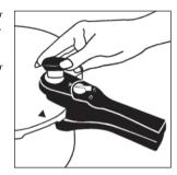
2. Move the open & close switch anti-clockwise fully to align the tail of the button with the "Close" position of the cooker on the lid handle. Refer to illustration.
