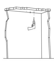
"Ensure the holes are drilled into a joist or other suitable mounting surface and not just into plaster."
