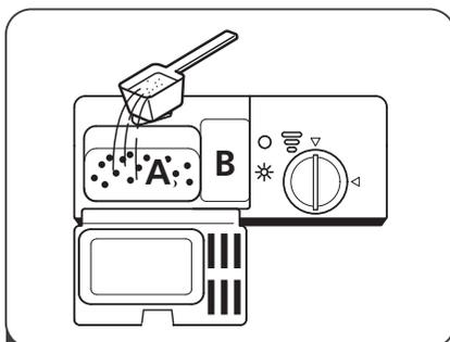
**2** Add detergent into the larger cavity (A) for main wash. For more heavily soiled wash loads, also add some detergent into the smaller cavity (B) for release during pre-wash.
