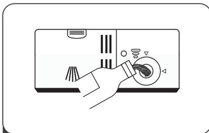
**2** Carefully pour in the rinse aid into the dispenser, whilst avoiding it to overflow.
