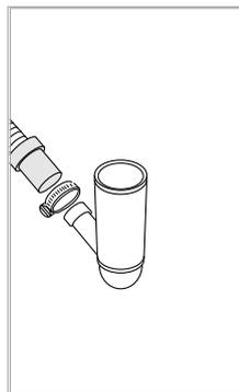
The hose must always discharge at least 350mm above the bottom of the machine. Attach the drainage hose with a hose clamp. Ensure that the drainage hose has no kinks.
