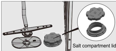
2. Place the funnel supplied with the dishwasher in the salt compartment top-up hole. First, pour in about 1L of water.
