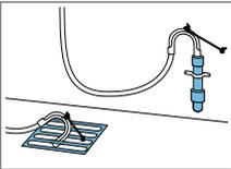
Fix and secure the water outlet hose with an elbow.
