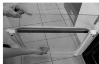
**Remove the centre glass taking care to support the weight of the glass when removing and fitting**
