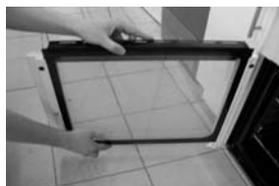
**Open the lower door and lift out the inner door glass**
