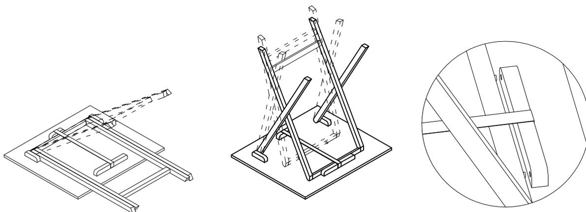
Warning - Please ensure that the wooden locating pins are in position before using the table .
