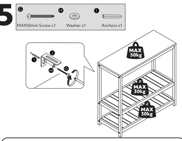
• WARNING: To prevent possible overbalancing this unit must be secured to a wall using the overbalance protector kit supplied.
