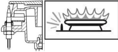
Thermal element activates the safety mechanism activates and cuts off the gas immediately against extinguishment of the top burners due to liquid overflow.
