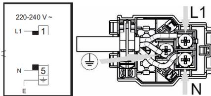
Connect the product to a grounded cable or line protected by a fuse according to the table of Technical Specifications. The manufacturer cannot be held responsible for any damages when used without grounding in accordance with the applicable regulations.
