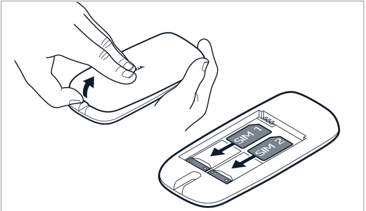
1. Put your fingernail in the small slot at the bottom of the phone, lift and remove the cover.
