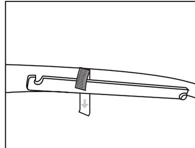
**NOTE:** Please loosen the lock as shown in diagram B, then close the canopy completely. After the canopy closed please secure the lock bar with velcro tape as shown in diagram C.
