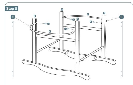
Finally, attach plastic rail **E** to legs using the 2 x 15mm screws **H**.
