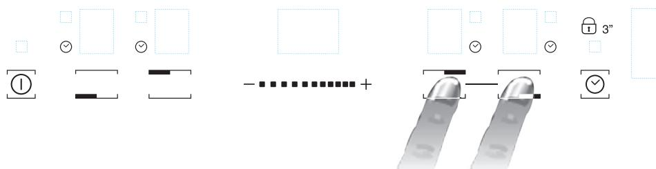
To change the power level (from 1 to max. 9 or P) press the -/+ buttons or slide your finger horizontally on the slider. To deactivate the HD FLEXI function, press simultaneously the 2 selecting buttons of the zones. To switch off the zones instantly, hold one of the zone selection button for 3 seconds.
