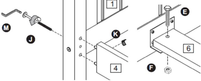
Step 7: Attach footend posts to side rails (8) using hardware parts J, K and M, then fix the centre rail (6) using hardware parts E and F with a spanner (not provided).
