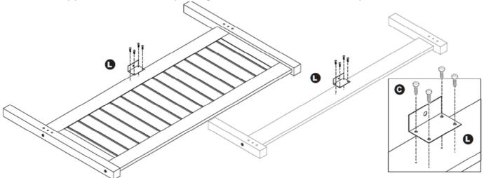
Step 6: Attach the side rails (4) to the headend posts using hardware parts J, K and M, then fix the centre rail (6) using hardware parts E and F and a spanner (not provided).
