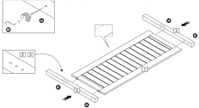
**Step 4**: Attach the left footend post (9) and right footend post (10) to the footend panel (8) using hardware parts H and M.
