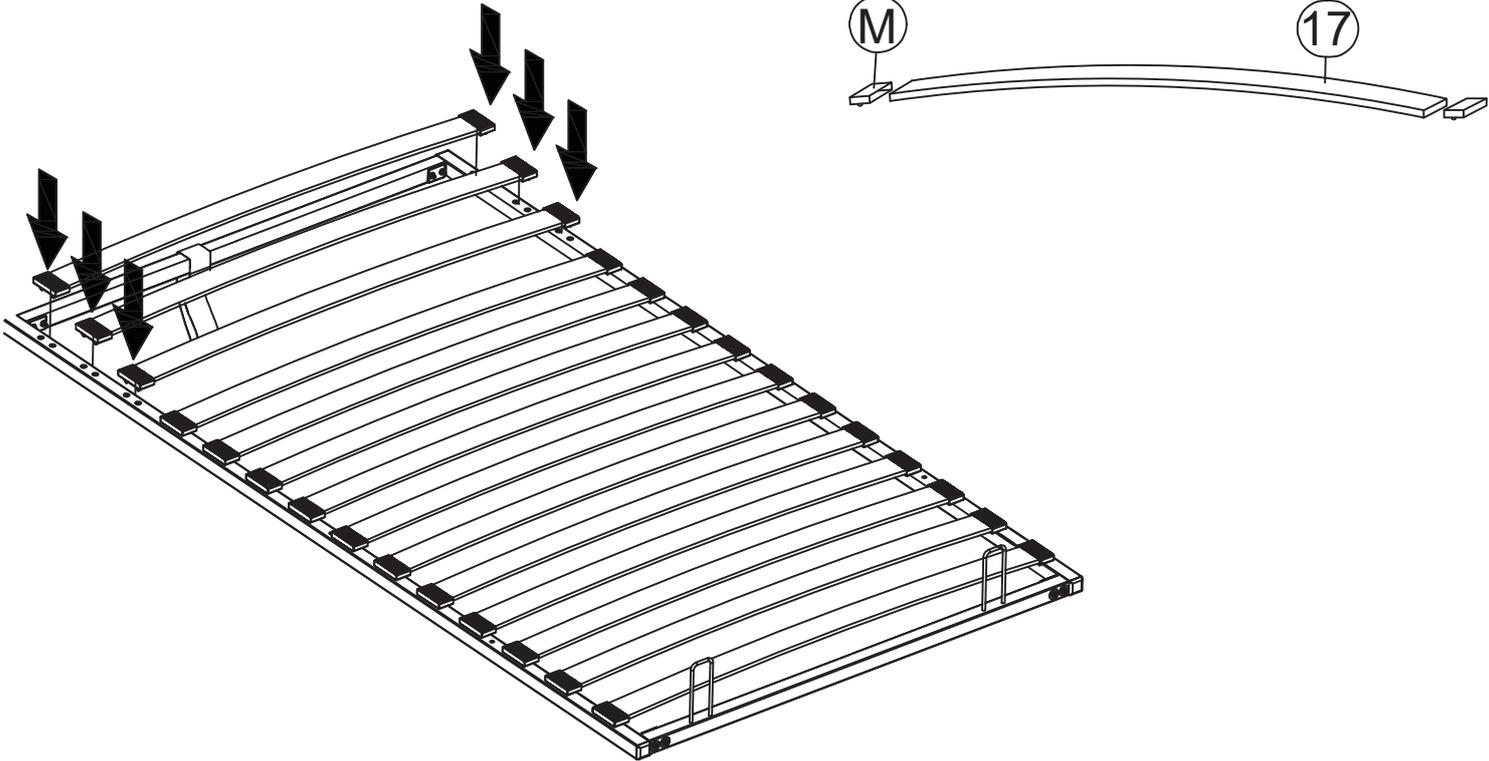
Step 10: Assemble the bed base on the right & left hydraulic frame and fix bolts starting from '1' to '3' as shown .
