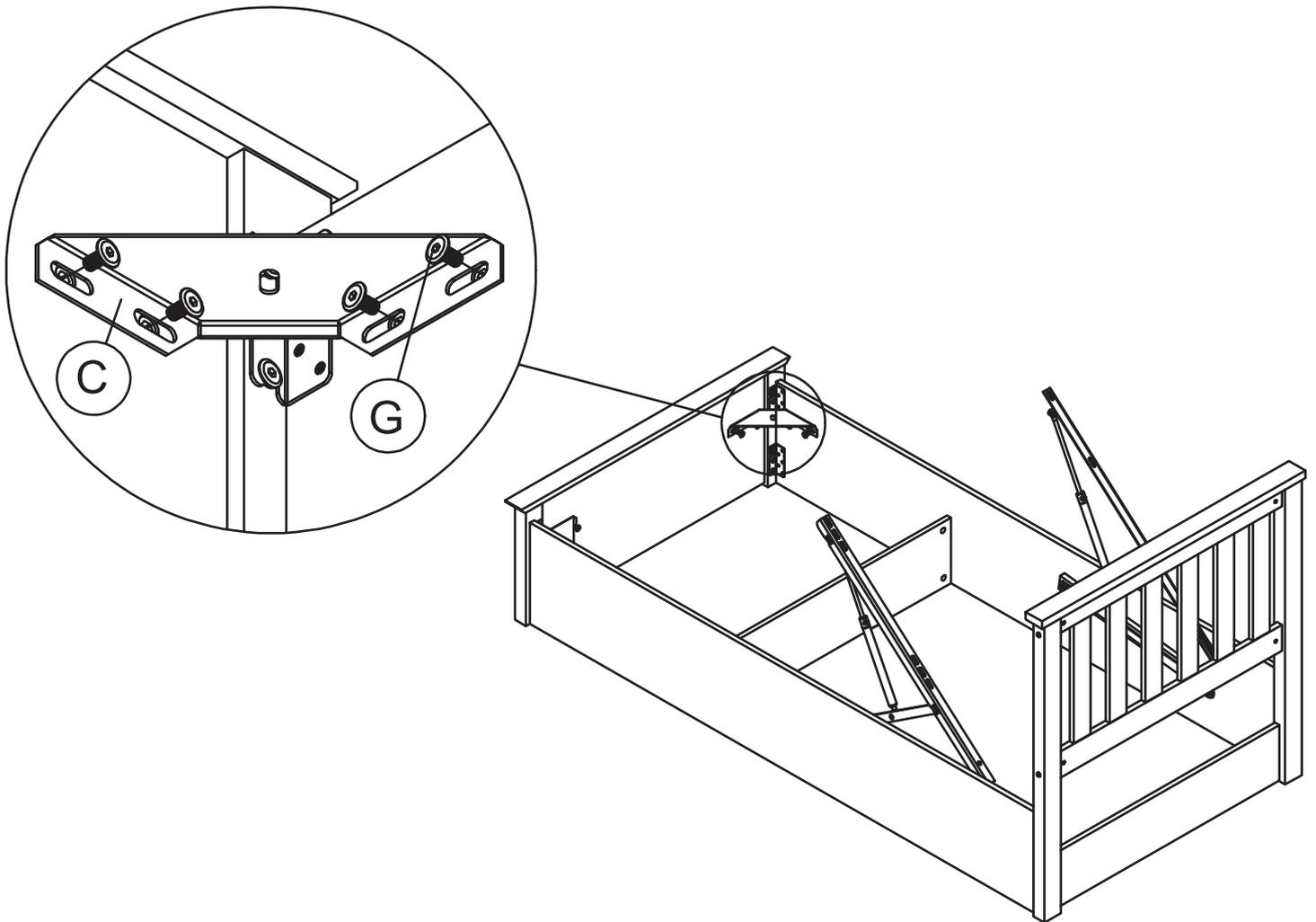
Step 8: Join together all the bed base parts (11),(12),(13) and (14) using hardware parts G,X & R and also slide part P onto Part 14 before bolting together. And then attach hardware parts J as shown. Important note: Please assemble follow arrow direction.
