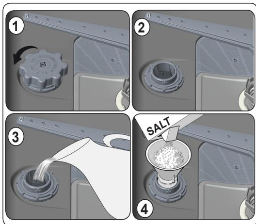
**Fill the salt compartment with water the first time you fill the salt compartment only.**
