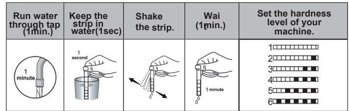
**NOTE:** Level is set 3 as default. If the water is well water or has a hardness level above 90 dF, we recommend that you use filter and refinement devices.
