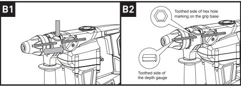
into the handle. Slide the depth gauge until the distance between the depth gauge end and the drill bit end is equal to the depth of hole/screw you wish to make.. Release the locking button to tighten.
