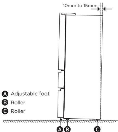
Rotate the adjustable feet clockwise to raise or raise counter-clockwise to lower your refrigerator. To make sure that the doors close
