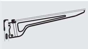
2. To reinstall a shelf, gently slide the shelf back into the refrigerator compartment, and then lower the shelf onto the rail support.
