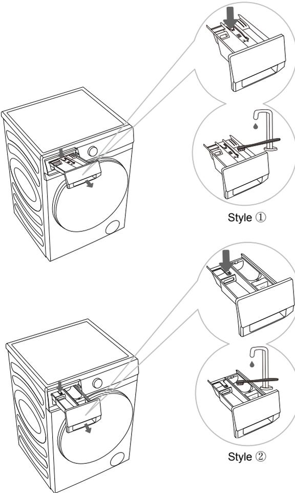
**1** To remove the detergent compartment from the housing, press the small tab.
