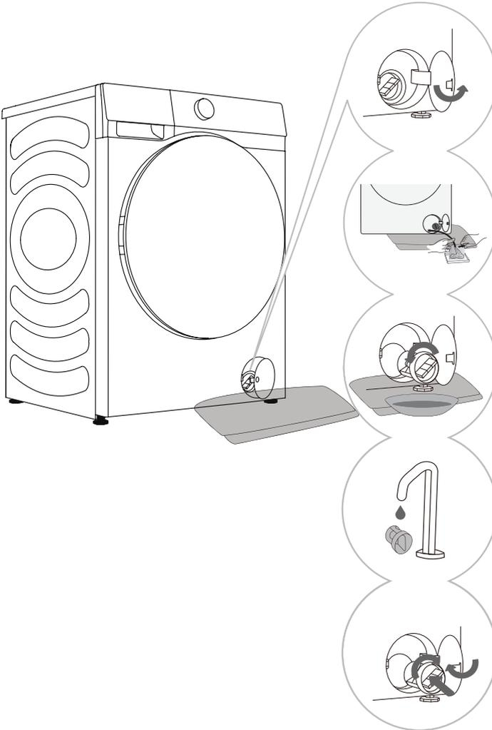
**1** Open the pump filter cap.
