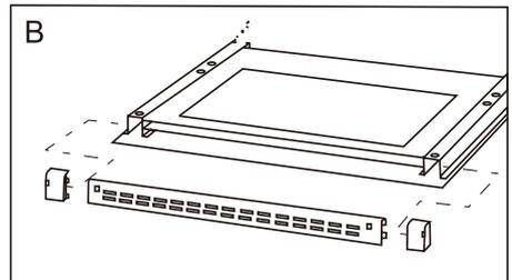
c. The inner glass pulled out from beneath plastic fixed block. After cleaning, the inner glass insert the following plastic fixed block, then install the above plastic mounting block .
