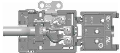
For 220V-240V earthed one phase connect on: Brown wire connect to L and blue wire connect to N, safety wire (Yellowgreen) connect to  $\oplus$
