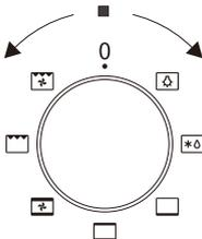
as well as the temperature regulator knob - to set a required function you should turn the knob to the selected position.
