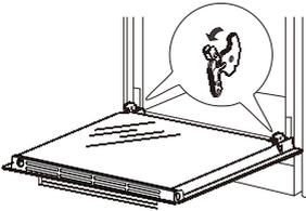
c. Gently close the oven door until you hear the sound of engagement, once they reach a clamping position, with both hands holding the door and continue to push, pull up at the same time so that the hinge bolt removed from the oven
