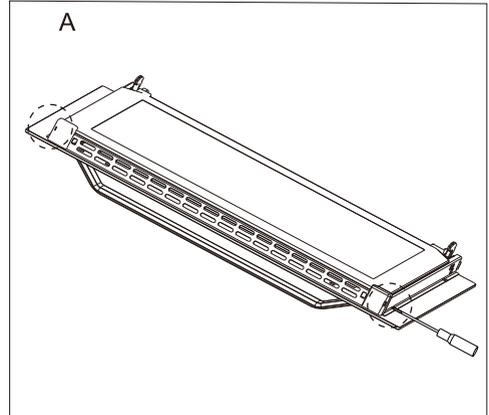
b. Remove the fixed block and the top ends of the plastic ventilation grid.
