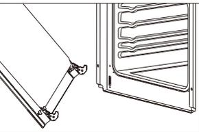
a. After cleaning, the hinge is aligned with the oven door latch push until bite each other
