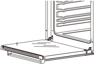
b. The latch hinges completely lifted.
