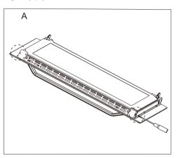
**b**.Remove the fixed block and the top ends of the plastic ventilation grid.
