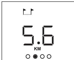
KM or MI ▶ Distance travelled during the session in kilometres or miles. This information is approximate: it does not take into account the resistance value, set by turning the brake knob.
