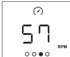
RPM Pedal revolutions per minute. When exercising, the value displayed is instantaneous. during a break, the value displayed is the average since the start of the session.
