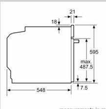
measurements in mm
