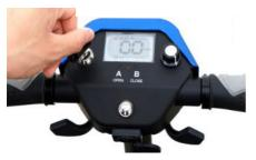
Step 2: Press the A-Open button on the control panel for 5 seconds and then release it. The buzzer will sound continuously, indicating that the control is ready to pair to the key fob.
