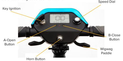
The scooter features an LCD display (right). The Speedo shows the current speed of the scooter.
