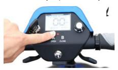
Step 3: Press both the A and B buttons on the key fob, at the same time. The buzzer will sound 5 short beeps, indicating that the control has paired with the key fob. The buzzer will then continue to sound.
