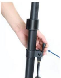
To adjust the tiller angle; Press the lever (arrowed) whilst pushing or pulling the tiller to the correct angle for the user. Release the lever to lock the tiller in position.
