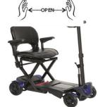
Note: You can fold or unfold the scooter manually by releasing the red manual fold release lever. If this is performed, then the opposite action should also be performed manually to reset. Failure to do so will not damage the scooter, but the autofold function may not work until the folding mechanism is manually reset. For this reason, it is recommended the manual operation is performed in emergency only.
