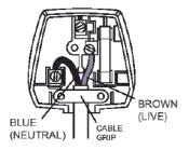
As the colours of the wires in the mains lead of this apparatus may not correspond with the coloured markings identifying the terminals in your plug, proceed as follows:
