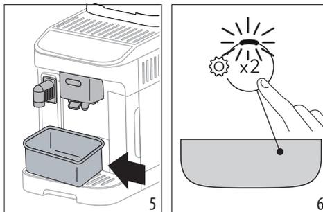
5. Press the button (x2) (fig. 6): the internal water circuits start to fill and the appliance will release hot water from the water spout.
