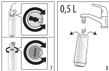
2. To activate the filter, run drinking water through the hole in the centre of the filter until water comes out of the openings at the side for more than a minute (fig. 8);
