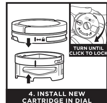
Align the yellow arrow on the side of the cartridge with the yellow arrow on the side of the dial cover, then insert the cartridge into the dial. Rotate the cartridge clockwise to lock it in place.
