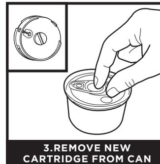
Remove the new Anti-Odour cartridge from the can. To maintain the life of the cartridge, keep it in the can until you are ready to install it.
