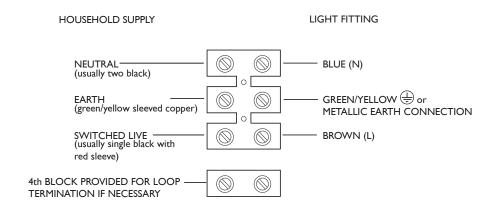
Please note: A fourth connection block is provided should you need it to make loop connection. If used in this way, insulate this block from the fitting and the other wires
