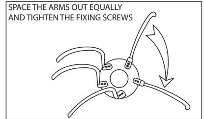
SPACE THE ARMS OUT EQUALLY AND TIGHTEN THE FIXING SCREWS
